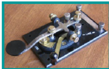
A telegraph machine used to send Morse Code messages.
